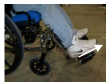
Improper support 2" gap between shoe & footrest
